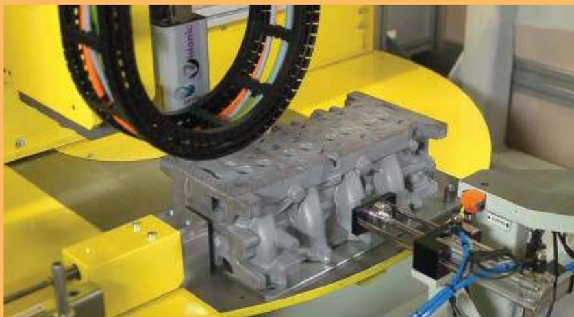
Groupe Visionic has developed an automated machine to measure features of engine blocks such as the depth and width of bore holes using laser distance sensors.
