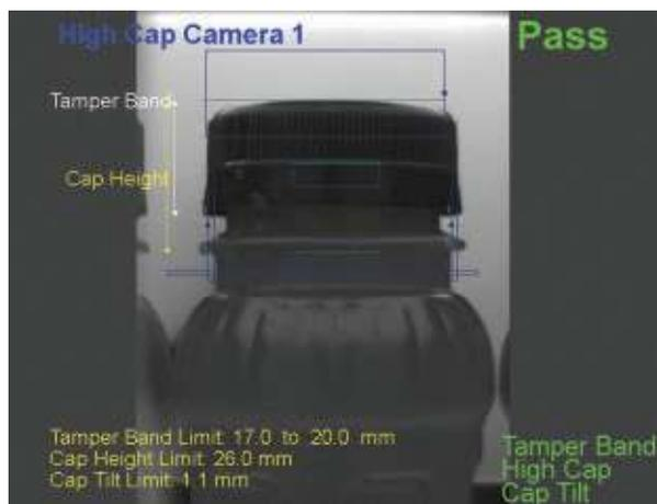
Measurements such as the distance from the cap shoulder to the tamper band (or pull-up), cap height measurement and the cap height are determined using Cognex's In-Sight Explorer software.
