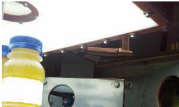
EPIC Systems has developed a system to inspect 6oz plastic bottles of fruit juice at speeds of up to 900 units per minute.
